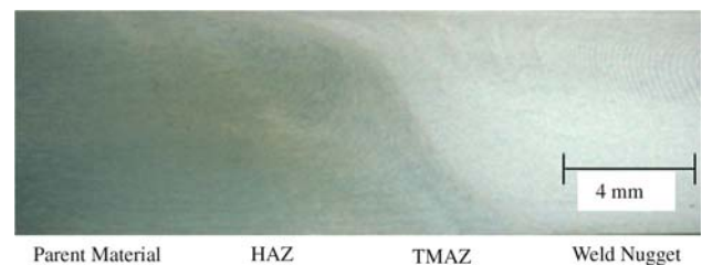
Fig. 3 A cross section of the welded specimen
